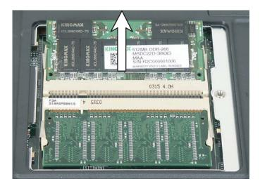
**8** Hold the new or replacement module at a 30-degree angle and press it into the empty memory slot. This module is keyed so it can only be inserted in one direction. If the module does not fit, make sure that the notch in the module lines up with the tab in the memory bay.
